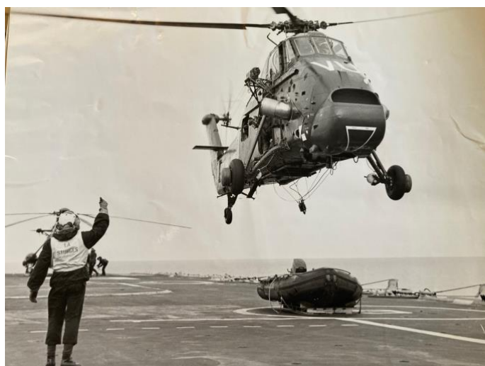
Directing Helicopter underslung pick up of Royal Marine Inflatable Raiding Craft Circa 1980/81
